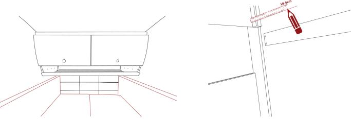
**3.** Measure from the floor of the camper and NOT the grid. Draw a line at 61cm from the 18.5cm mark and measure again 61cm about 40cm from the first mark. Use the leveling rule and draw a line between those 2 points. Repeat on opposite side.
