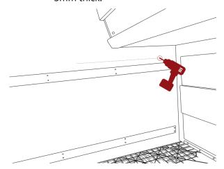
**5.** Place the rail(L/R) and then place the screw in the first hole. Before it is fully tightened, adjust the predrilled hole with markings with your line. Now mark the 5 remaining holes and drill as previous described. Repeat on opposite side.
