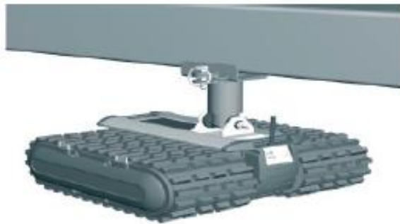
Illustration of the Robot Trolley mounted on the side members of the caravan:
